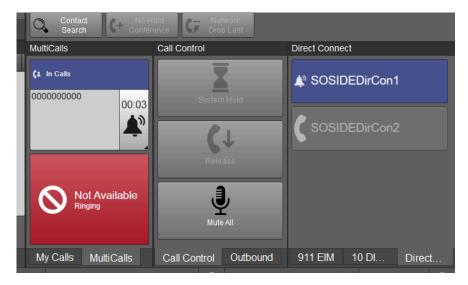
This is a screen shot of what the call taker will see when a line that comes in on direct connect. The line rings in on the direct connect tab and is purple.
